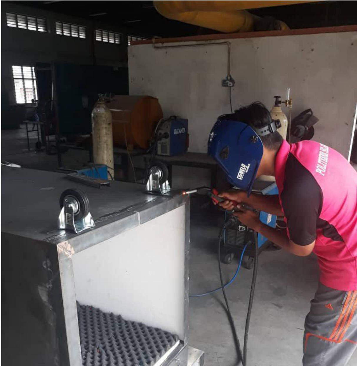
*Figure 3.3.3 Welding the wheels behind the Sieve O' Sound*
