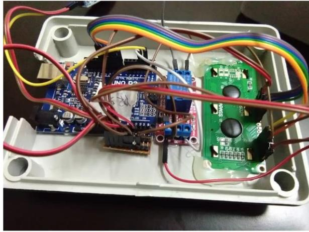
Diagram 3.5.1.2 shows the jumper cables have been installed to the other electrical components
