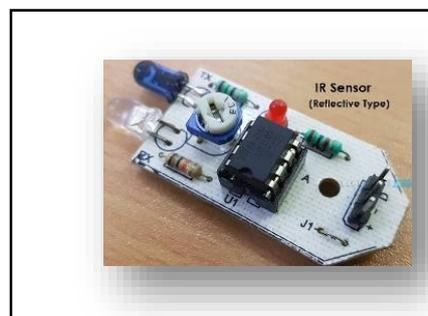
Diagram 2.2.2.3 Infrared Sensor
