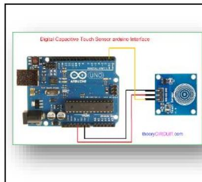
This device uses your body as part of the circuit. When you touch the sensor pad, the capacitance of the circuit is changed and is detected. That detected change in capacitance results in the output changing states. It is suitable to detect capacitive element variations. It consumes very low power and the operating voltage is only between 2.0V~5.5V.
