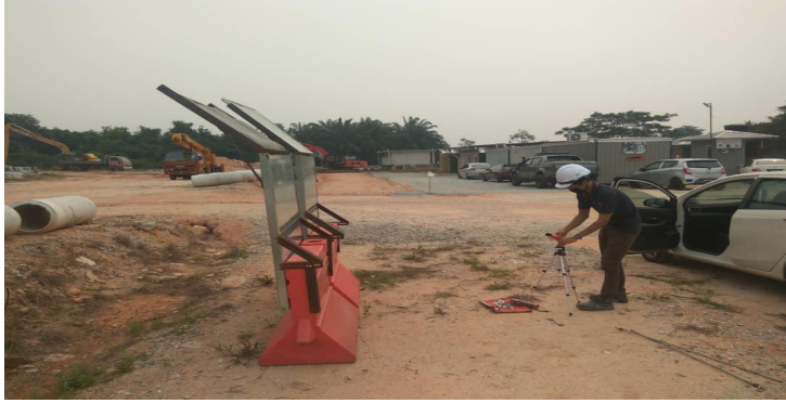
Figure 9 shows taking a reading behind panel (500mm)
