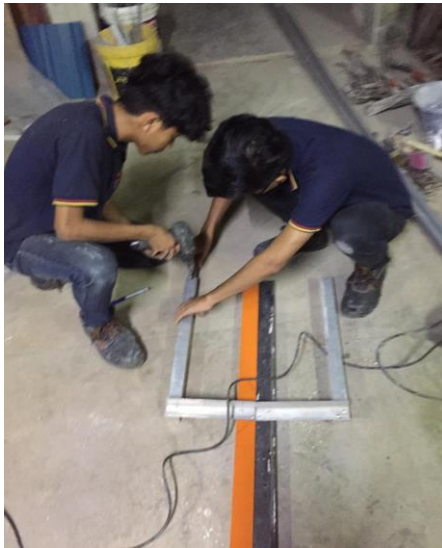
Figure 3.4.1 v : Cut the iron, measure, puncture and drill
