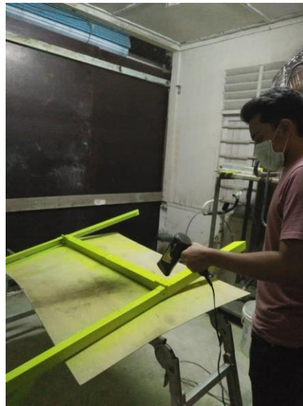
Figure 3.4.1 vi: Cut the wood, drill the hole and painting the panel frame.
