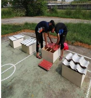
Figure 3.10: apply the roof on the house model.
