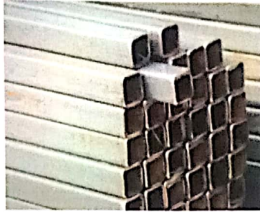
Figure 3.12 Mild steel hollow
