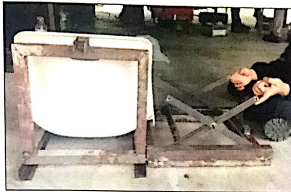
Figure 4.4 Base and back frames with 'X' scissor lift
