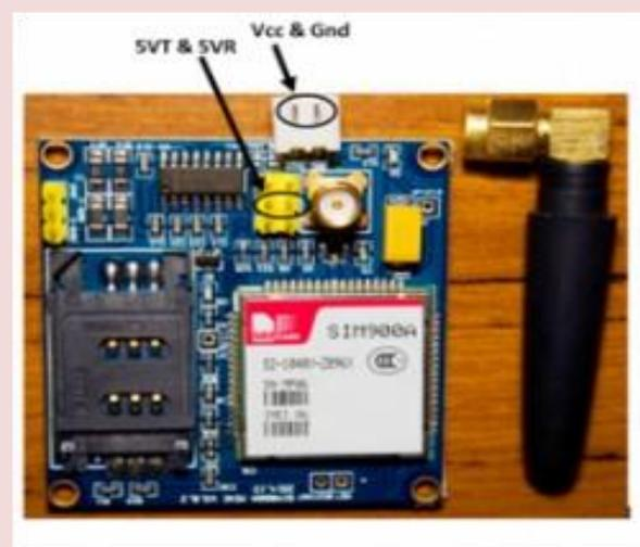
Figure 5: The GSM modules
