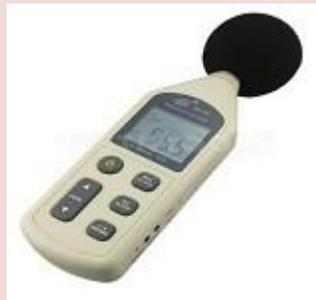
**Figure 1: Sound Level Meter Equipment**
