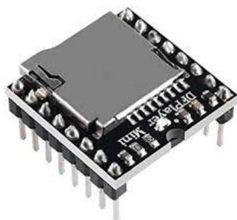
The DFPlayer Mini MP3 Player For Arduino is a small and low price MP3 module with an simplified output directly to the speaker. The module can be used as a stand alone module with attached battery, speaker and push buttons or used in combination with an Arduino UNO or any other with RX/TX capabilities.
