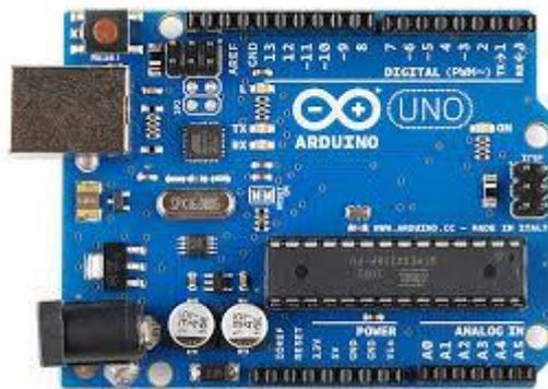
Arduino Uno is a microcontroller board which is an open-source electronics platform mainly based on AVR microcontroller. It allows the designers to control and sense the external electronic devices in the real world. It has 14 digital input/output pins, 6 analogue inputs, a 16 MHz quartz crystal, a USB connection, an ICSP header and a reset button, a power jack.
