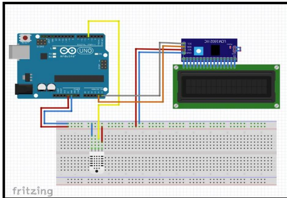
Figure 3. 6: Circuit of Prototype Development
