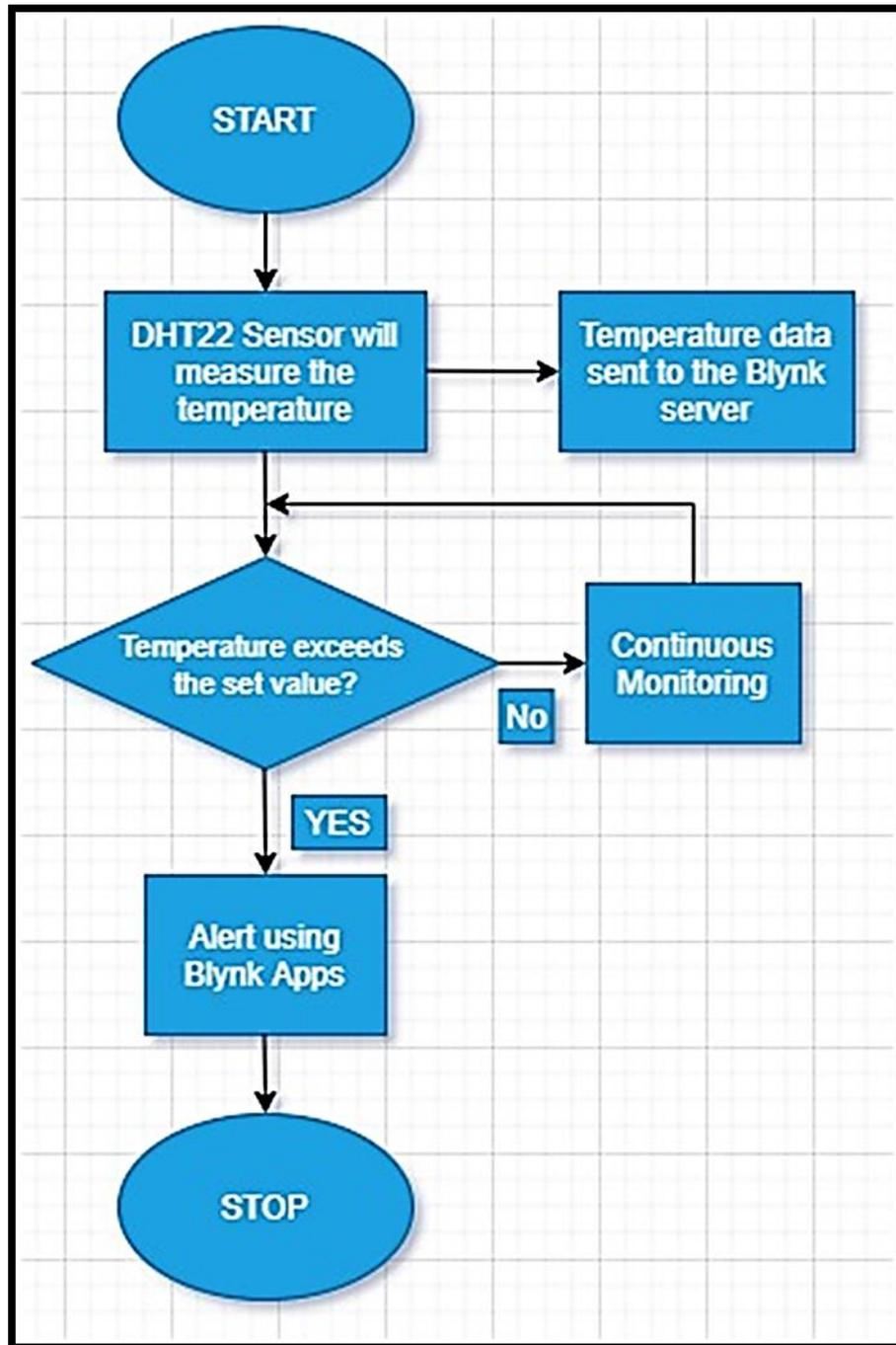
Figure 3. 2: Flow chart of operation of the system
