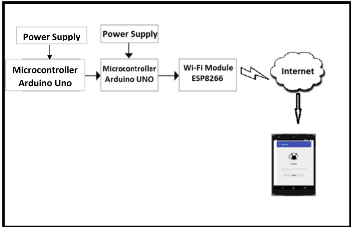
Figure 3. 2: Block diagram of the Project
