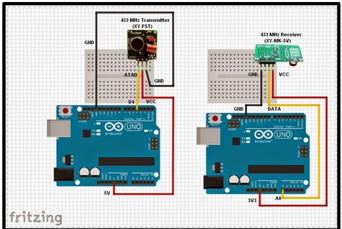
Figure 3. 6: Circuit of Prototype Development
