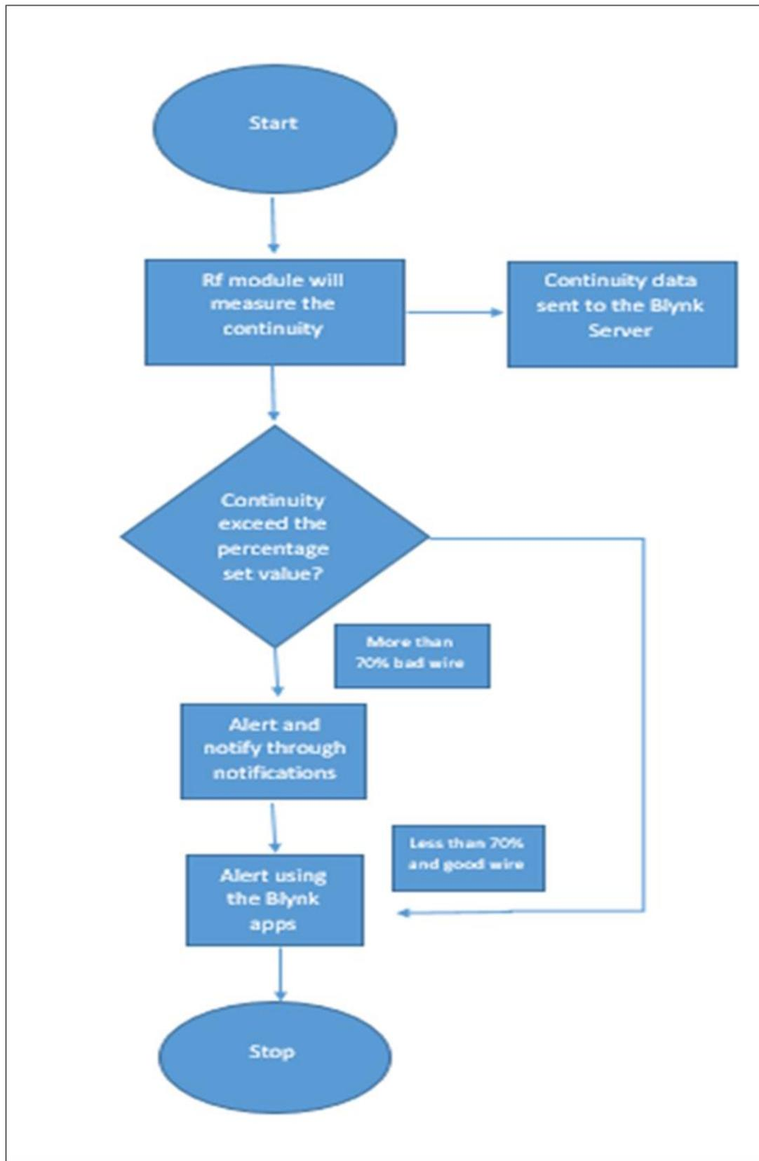
Figure 3. 2: Flow chart of operation of the system
