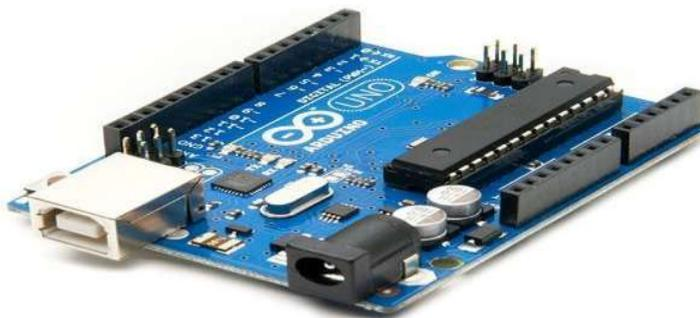
**Arduino Uno** is a microcontroller board based on the ATmega328P (datasheet). It has 14 digital input/output pins (of which 6 can be used as PWM outputs), 6 analog inputs, a 16 MHz quartz crystal, a USB connection,
