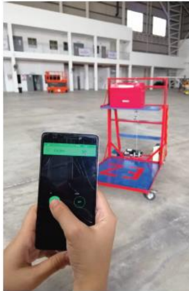
Figure 5: Mobile app Blynk to operate EZ Lifter
