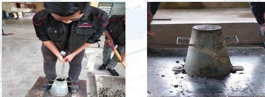
Figure 2: Compact concrete by using tamping rod
