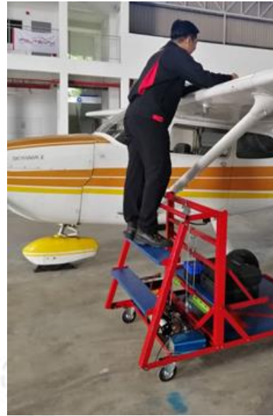
Figure 6: User testing the EZ Lifter for Cessna 172 maintenance work.
