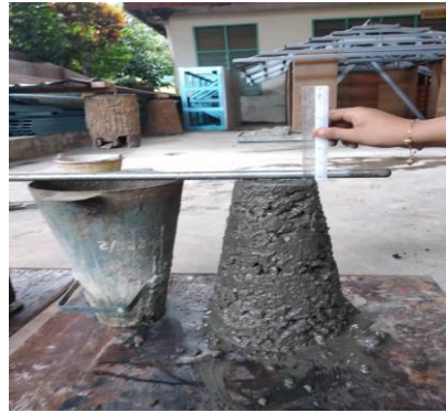
Figure 4: The slump is measured by using the upturn cone and tamping rod as a guide
