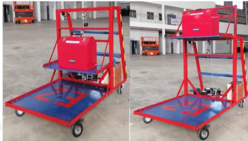
Figure 1: The EZ Lifter on normal operation (left) and lifting operation (right)
