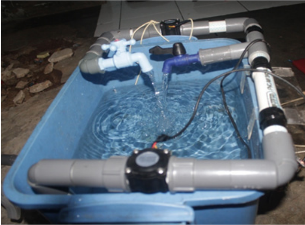
Fig. 12. Simulation of water discharge and leakage measurements
