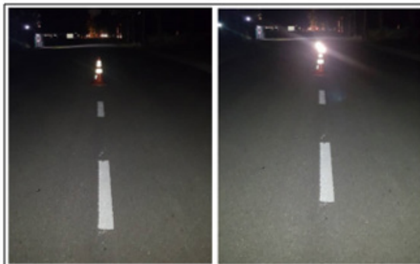
Fig. 10. Comparison between existing safety cone (left) and FEFL (right) for a 10 meter view
