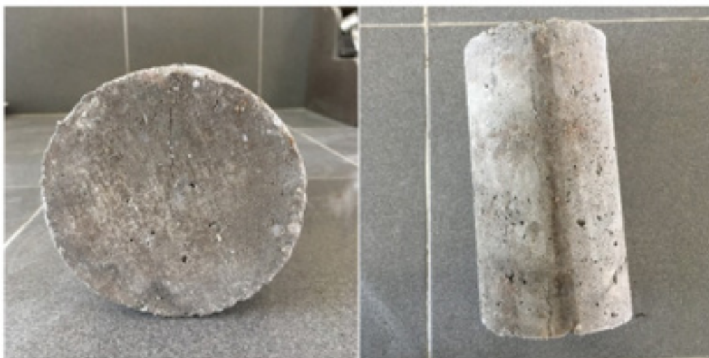
Fig. 7. Normal Weight Concrete of cylindrical specimen cracking behaviour
