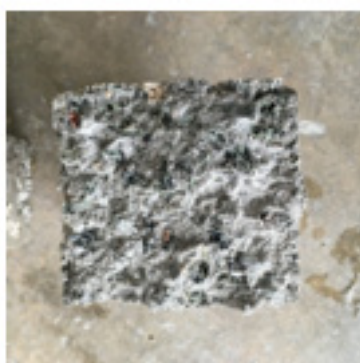
Fig. 4. Cross section of the specimen of POCLC
