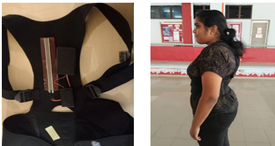
Fig. 3. Above pictures shows where the sensors are embedded in Support Vest.
