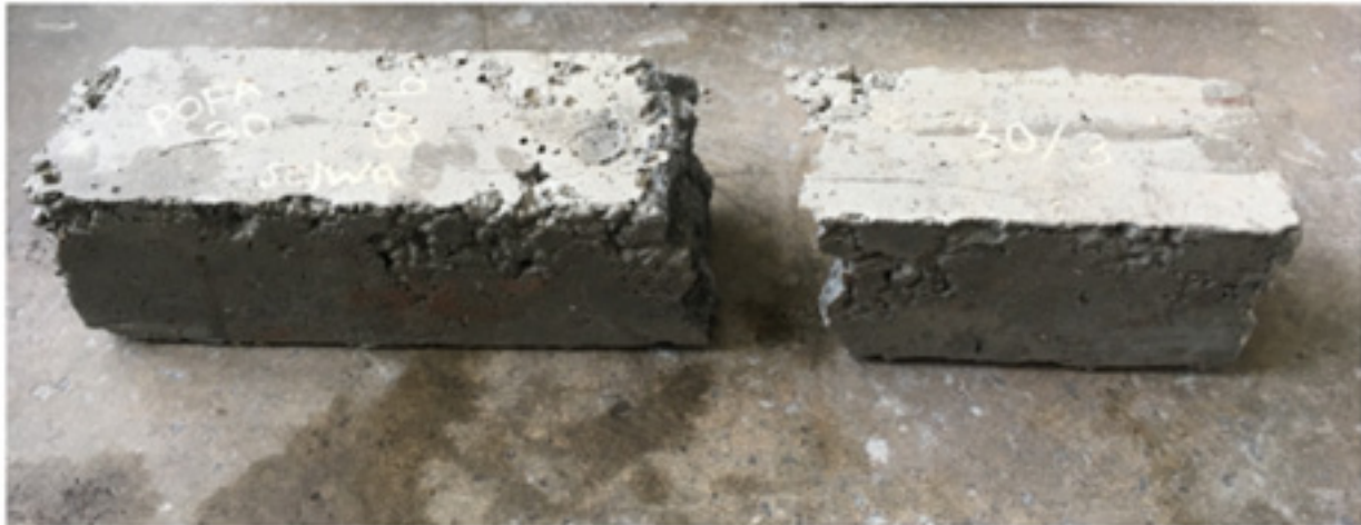
Fig. 10: Failure mode of POCLC concrete beam in flexure.
