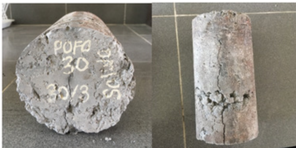
Fig. 8. POC Lightweight Concrete of cylindrical specimen cracking behaviour
