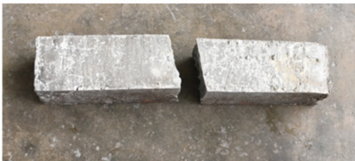
Fig. 9: Failure mode of normal weight concrete beam in flexure.
