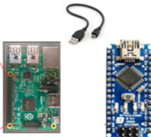
Fig. 9. Connection between Raspberry Pi 3 and Arduino
