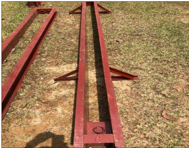
Figure. 7. Ground Beam Steel Formwork
