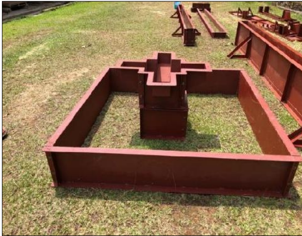
Figure 11. Pad Footing Steel Formwork
