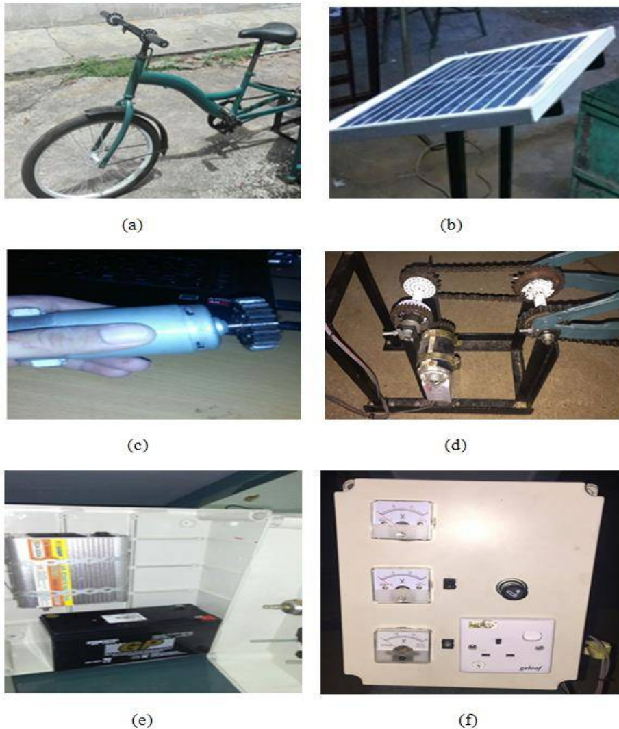
Figure 1: Component used in a hybrid solar bike (a) Bicycle, (b) Solar panel (c) Generator, (d) Gear, (e) Inverter and Battery and (f) Meter and socket plug
