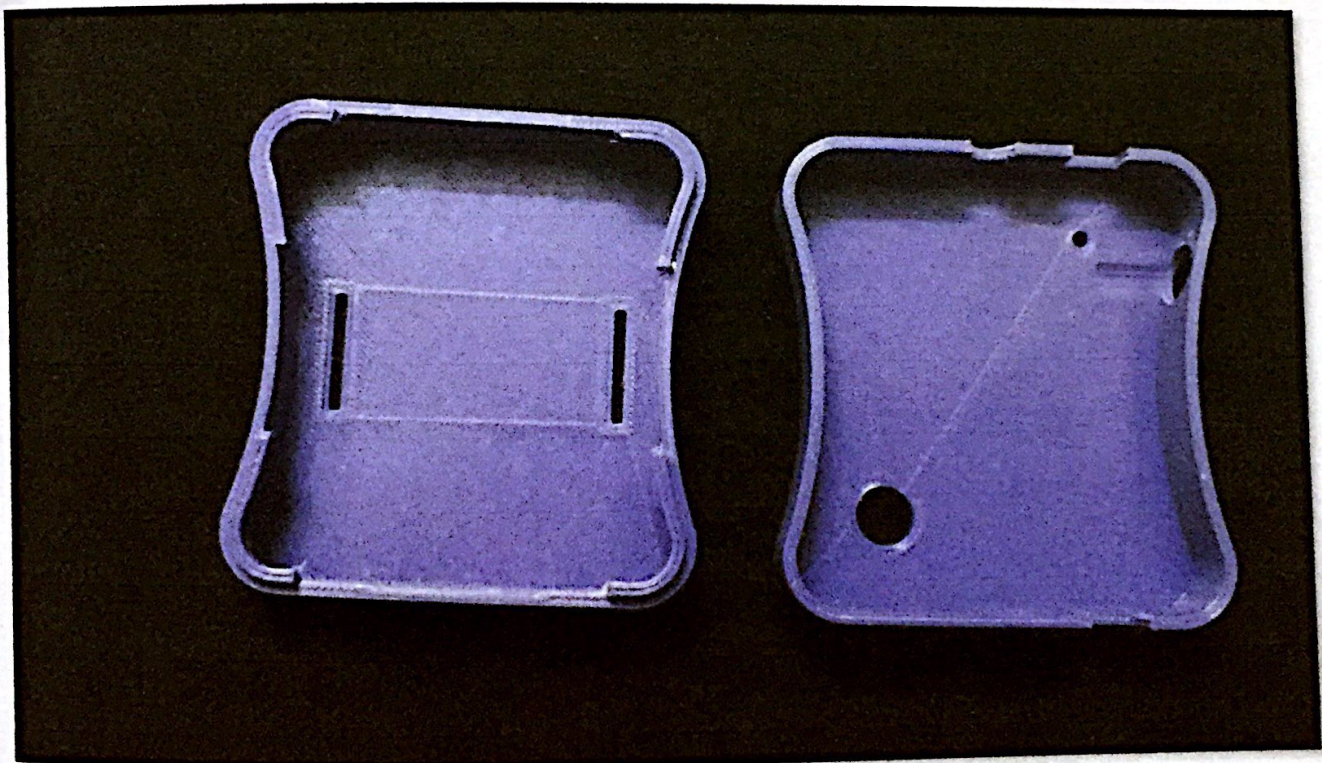
Figure 4.17: Back view of front and back part of housing
