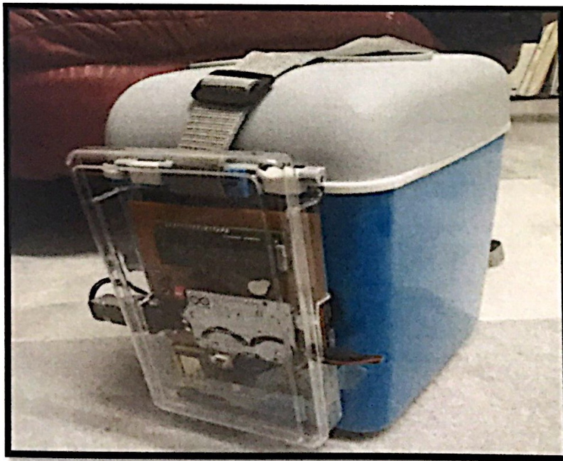
Figure 4.1: Prototype of Blood Cooler Transportation Box with GSM Technology
