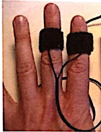
Figure 2.2: Sensor placement when measuring GSR on finger
