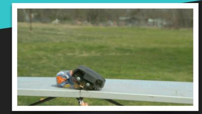
3. Generally, the complete inflation of airbags of a vehicle takes approximately 30 millisecond
