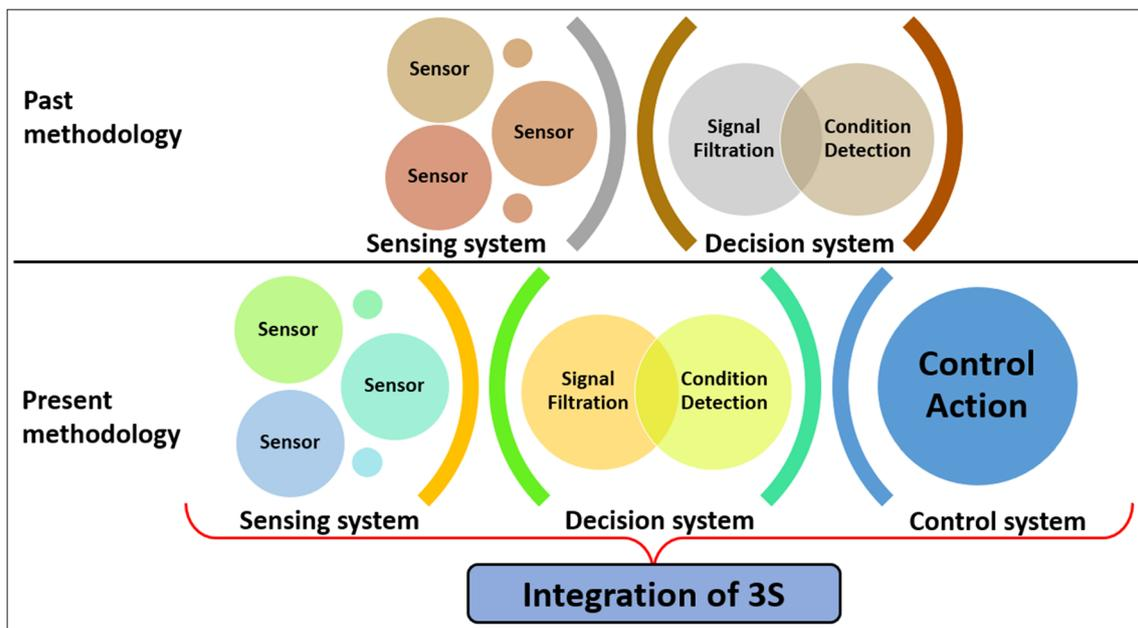
Fig. 3 Methodology of past and present machine process condition monitoring
