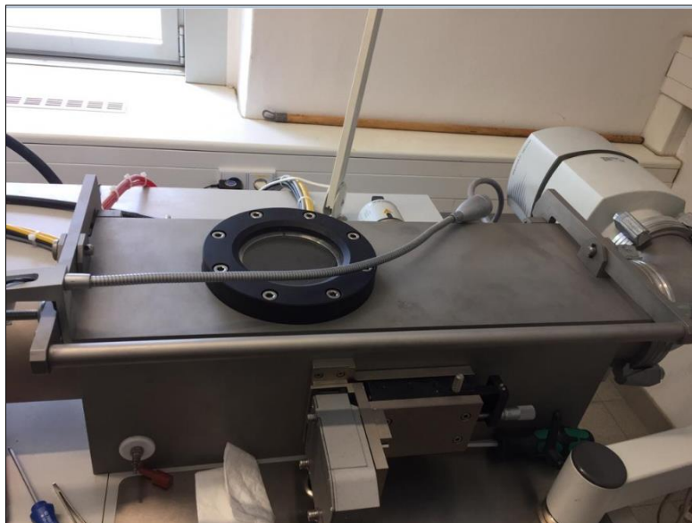
Figure 2. Quenching and deformation dilatometers.
