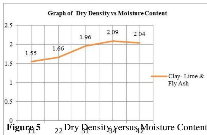
**Figure 5** Dry Density versus Moisture Content
