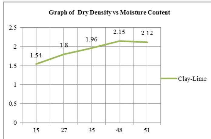
**Figure 4** Dry Density versus Moisture Content
