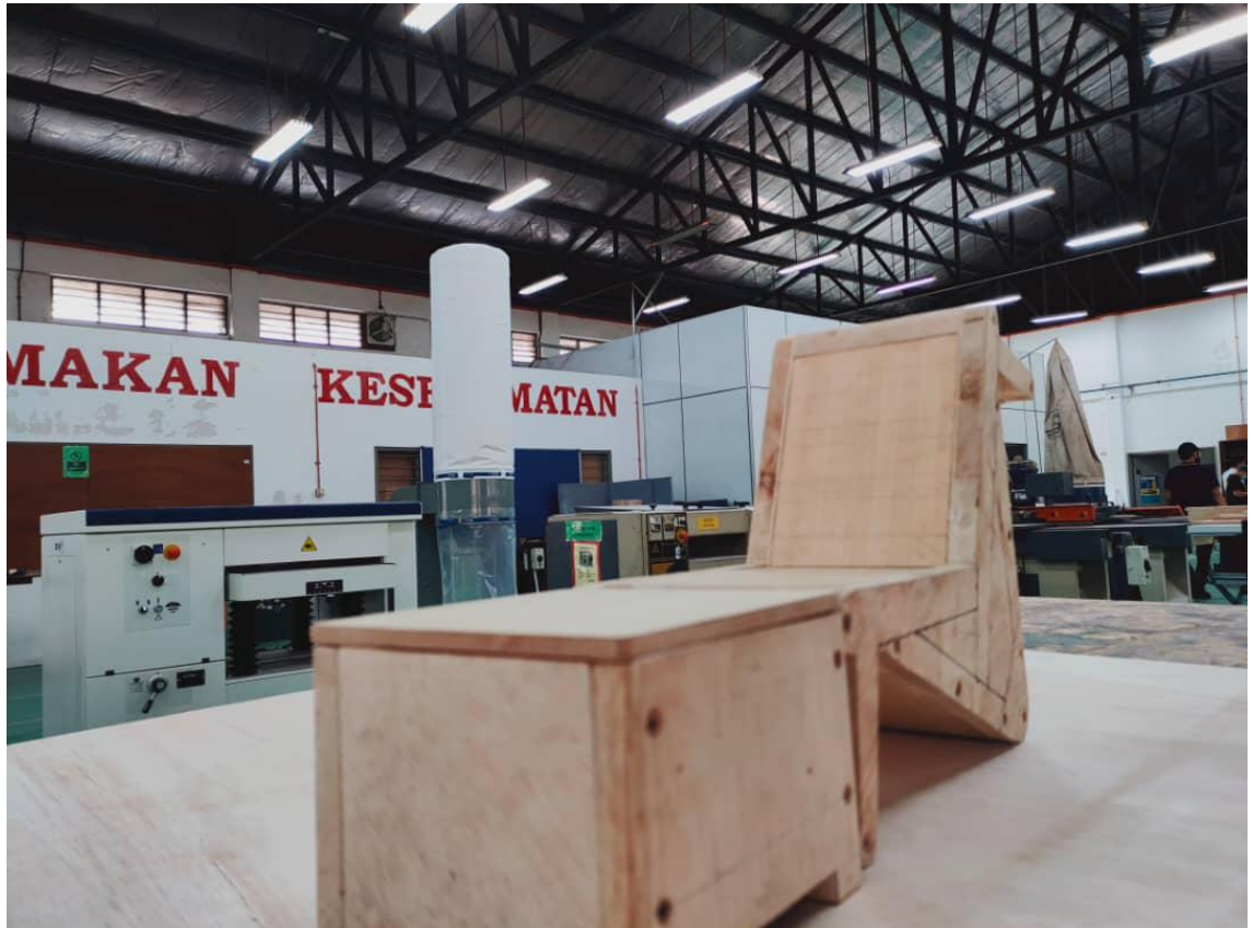
Image 4. Create Ohsuga Model using Blockboard scale (1:5) "Sofa bed view"
