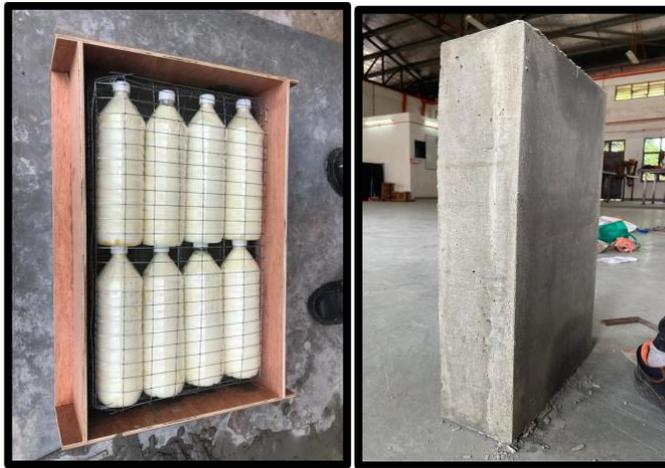
Figure: lightweight wall panel prototype has been replaced with bottle plastic filled with foam (pu200) as a brick
