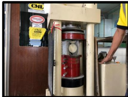
Figure: Testing of water absorption and compressive strength on lightweight wall panel
