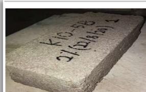
After 24 hours, the brick is taken out from the mould.
