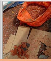
Crushing the clay roof tiles into grain size particles.
