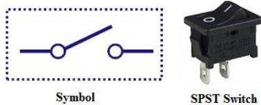
This is the basic ON and OFF switch consisting of one input contact and one output contact. It switches a single circuit and it can either make (ON) or break (OFF) the load. The contacts of SPST can be either normally open or normally closed configurations .
