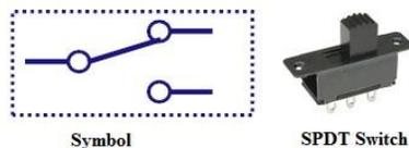
This switch has three terminals, one is input contact and remaining two are output contacts. This means it consists of two ON positions and one OFF position. In most of the circuits, these switches are used as changeover to connect the input between two choices of outputs. The contact which is connected to the input by default is referred to as normally closed contact and contact which will be connected during ON operation is a normally open contact.
