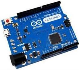
The Arduino Leonardo is a microcontroller board based on the ATmega32u4. It has 20 digital input/output pins (of which 7 can be used as PWM outputs and 12 as analog inputs), a 16 MHz crystal oscillator, a micro USB connection, a power jack, an ICSP header, and a reset button. It contains everything needed to support the microcontroller; simply connect it to a computer with a USB cable or power it with a AC-to-DC adapter or battery to get started.
