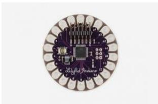
The LilyPad Arduino is a microcontroller board designed for wearables and e-textiles. It can be sewn to fabric and similarly mounted power supplies, sensors and actuators with conductive thread. The board is based on the ATmega168V (the low-power version of the ATmega168) (datasheet) or the ATmega328V (datasheet). The LilyPad Arduino was designed and developed by Leah Buechley and SparkFun Electronics.
