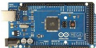
Arduino is an open-source physical computing platform based on a simple i/o board and a development environment that implements the [Processing/Wiring](#) language. Arduino can be used to develop stand-alone interactive objects or can be connected to software on your computer (e.g. Flash, Processing, MaxMSP). The open-source IDE can be [downloaded](#) for free (currently for Mac OS X, Windows, and Linux)
