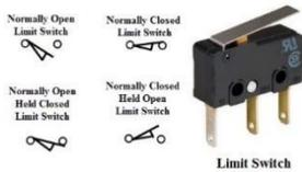
The control schemes of a limit switch are shown in above figure , in which four varieties of limit switches are presented. Some switches are operated by the presence of an object or by the absence of objects or by the motion of machine instead of human hand operation. These switches are called as limit switches. These switches consist of a bumper type of arm actuated by an object. When this bumper arm is actuated, it causes the switch contacts to change position.
