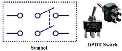
This is a dual ON/OFF switch consisting of two ON positions. It has six terminals, two are input contacts and remaining four are the output contacts. It behaves like a two separate SPDT configuration, operating at the same time. Two input contacts are connected to the one set of output contacts in one position and in another position, input contacts are connected to the other set of output contacts.
