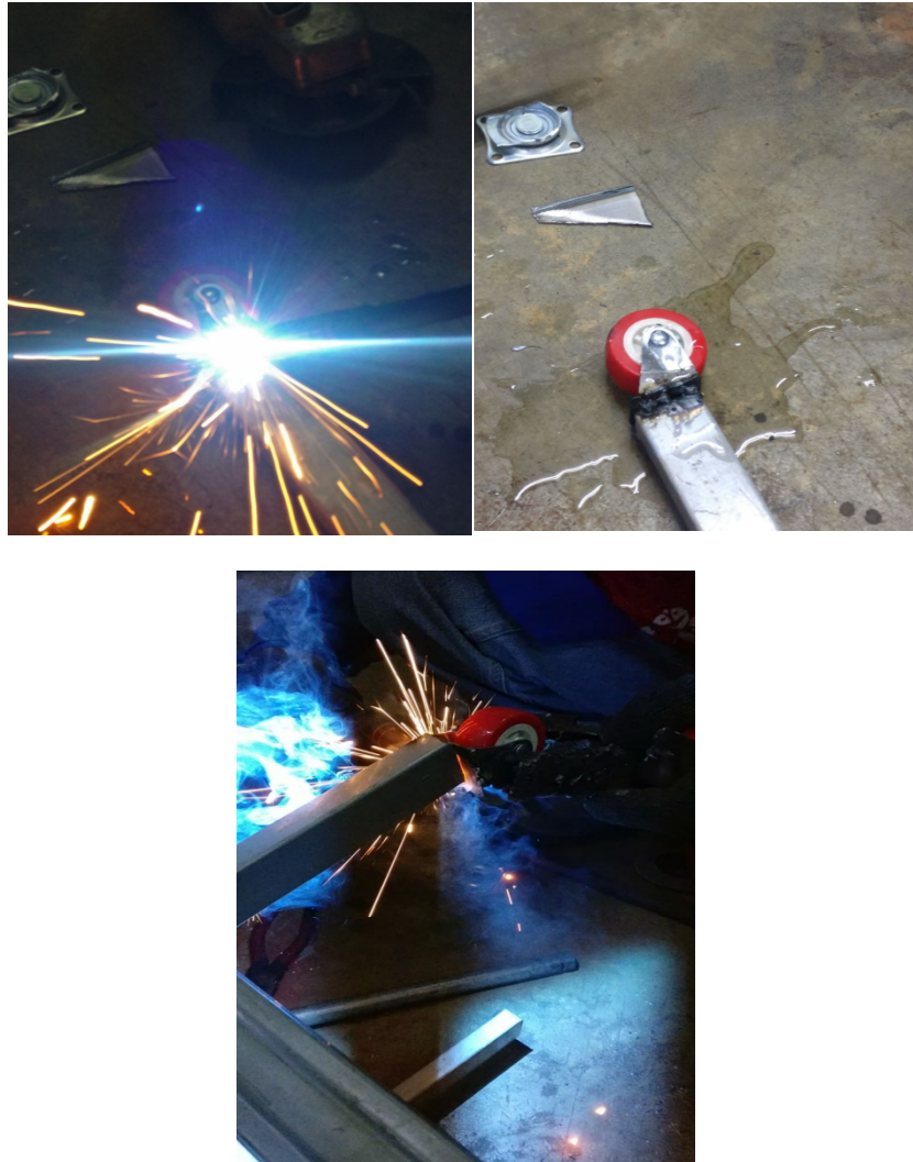
Figure 3.3 ( Installation of Wheels by using MIG welding)
