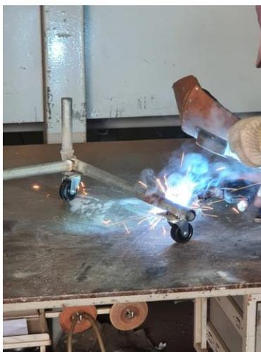
Figure 3.3.4(d): Welding process of the lower part / base / wheel of the wheel chair.
