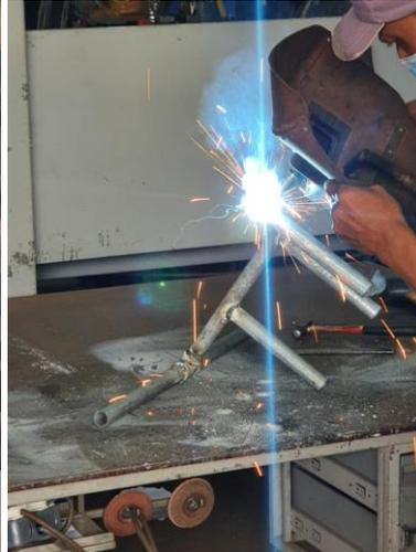
Figure 3.3.4(c): Welding process of the upper part / main frame of the wheel chair.
