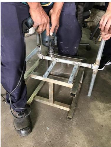
Figure 3.3.4(e): Drilling process of the seating area.
