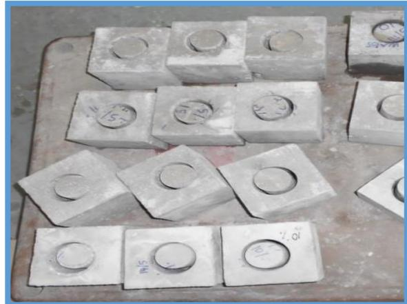
Figure 8.2. The concrete cores sample
