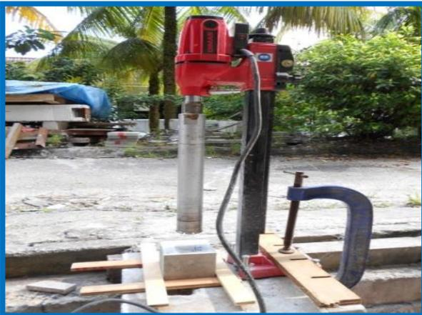
Figure 8.1. The coring machine
