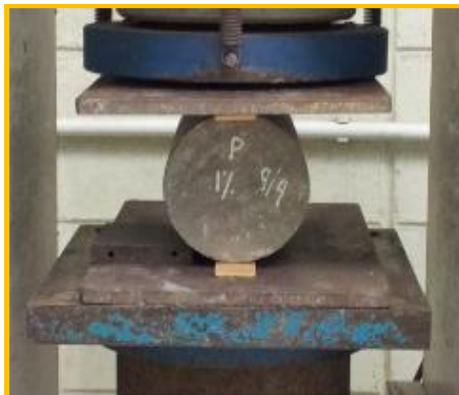
Figure 7.2. Testing for indirect tensile test
