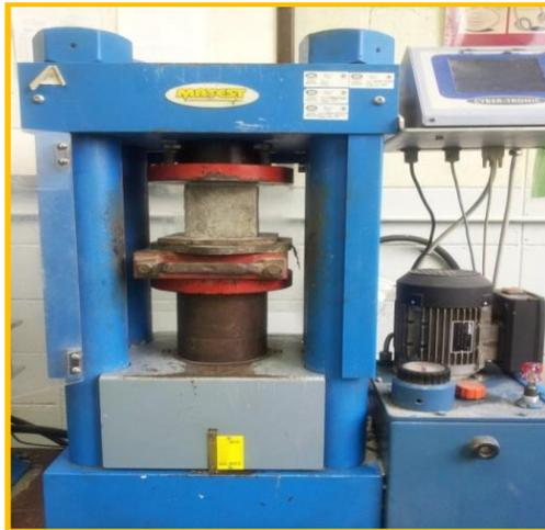
Figure 7.1. Testing for compressive strength
