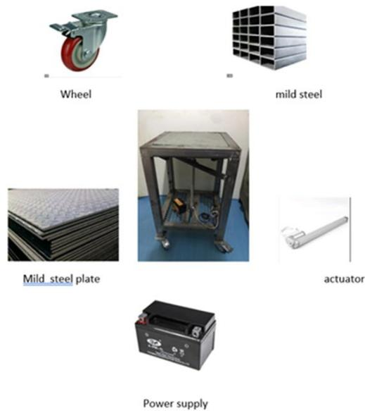
1. First of all, we cut stainless steel into 4 rods measuring 0.7 meters each to be used as table legs.
