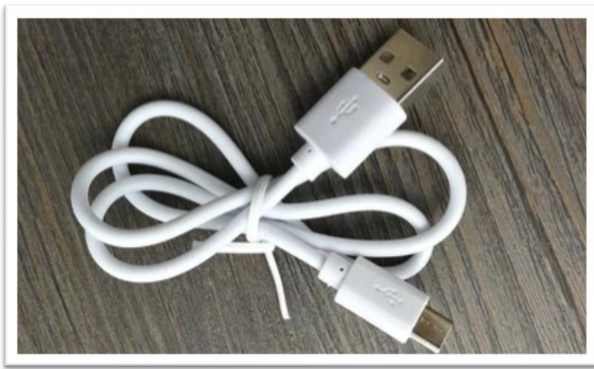
Figure 2.3.6- Mirco USB charge
