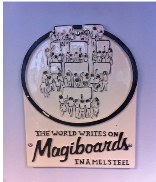
Figure 2.6 Door sign made of enameled steel
