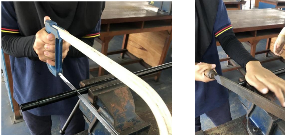
Figure 3.7 Cutting process using handsaw and file tool.
