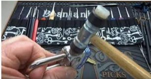
Diagram 2.2.2.1 shows padlock that hammered to unlock
