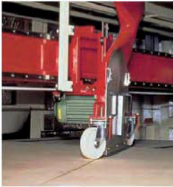
Figure showing diagonal saw for cut to length panels after continuous hot pressing (Metso Panelboard).
