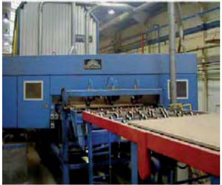
Figure showing diagonal saw for cut to length panels after continuous hot pressing (Metso Panelboard).
