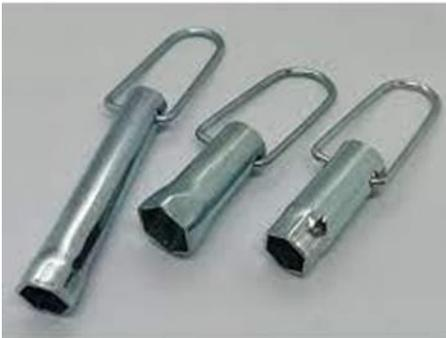
The most important tool is a spark plug socket. Spark plug sockets come in two sizes which is  $\frac{5}{8}$  and  $\frac{13}{16}$  inches. Most aftermarket spark plug sockets have a rubber insert that holds the plug in place.
