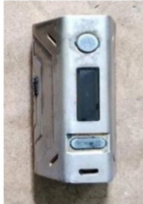
Figure 3.2.2 e) shows the Vape Device used as a heating device as the heat source of the cutting wire
