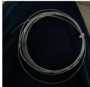
Figure 3.2.2 b) shows a Stainless Steel 316 used as cutting wire
