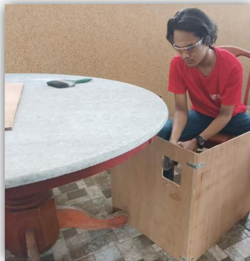
**the process of perforation on the wood plan for the space to place the exhaust fan**
