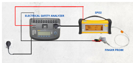
Figure 4.1: Connection Between Medical Equipment and Safety Analyzer
