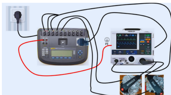
Figure 3 : Connection Between Medical Equipment and Analyzer
