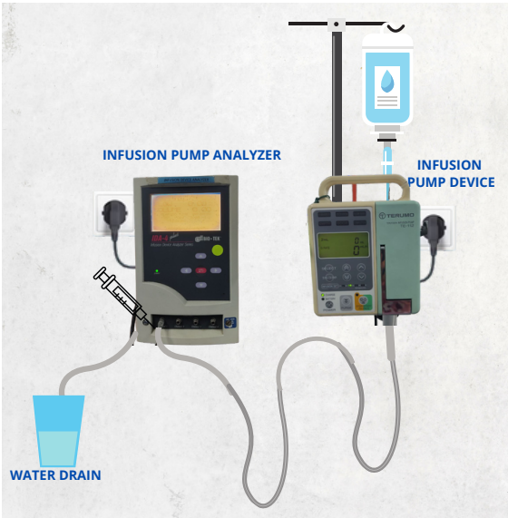
Figure 6: Connection Between Medical Equipment and Safety Analyzer
