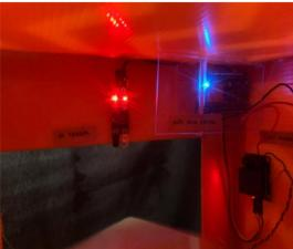
This project circuit was connected to WiFi/Hotspot and all the components was connected to power supply (Battery). The light from IR Sensor and Node MCU Esp8266 were working perfectly although it takes a few seconds delay to see the result. Output in the circuit are working properly. Light from Node MCU Esp8266 and IR Sensor will turn on both when the parcel is received in the mailbox.
