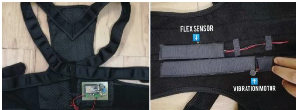
Figure 5. ESP32 circuit board with Flex Sensor and Vibration motor combined together
