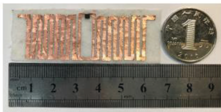
Figure 2: Fabricated Wearable RFID Tag Antenna on Cotton Fabric [25]
