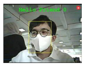
Figure 3.13 : ESP - 32 recognize user face
