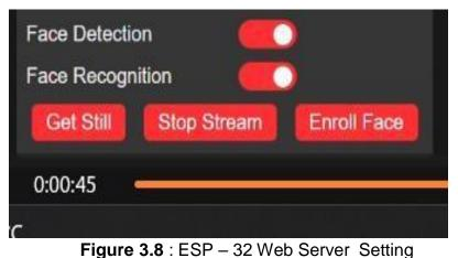
Based on figure 3.8, in the ESP -32 web server settings, press the enroll face button to scan theface so that the scanned face will be stored in the ESP -32 database.
