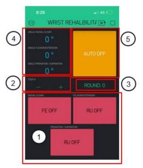
Figure 6: Interface of IoT implementation using Blynk application for controlling the movement of servo motor
