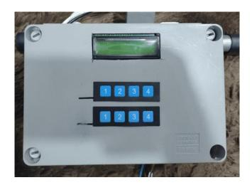
Figure 4: Keypad to control the speed
