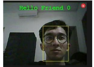
Figure 3.10 : ESP - 32 Camera recognize face
