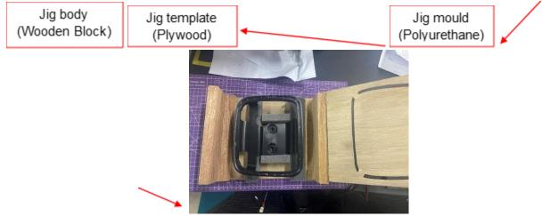
Figure 6: The jig prototype.
