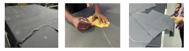
Figure 2.3: Manual marking & cutting
