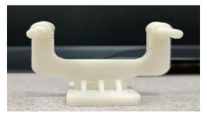
Figure 7: Checking jig that have been produced using rapid prototype
