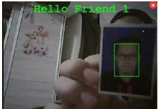
Figure 3.16 : ESP -32 detect the photo
