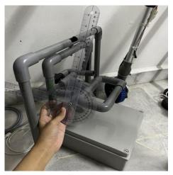
Figure 10: Measure the ROM of the device using goniometer Table 2: Comparison ROM of device between normal ROM of the wrist
