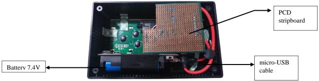
Figure 8. the inside of SMAD device
