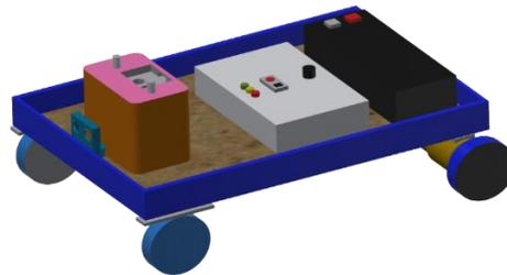
**Figure 4: Mechanical Design of Automated Fumigation using Tinkercad**
