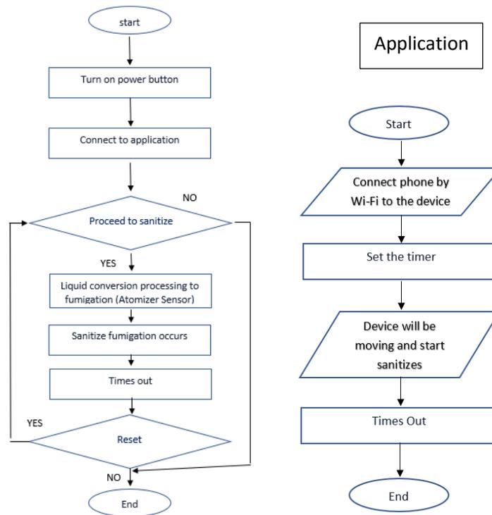
**Figure 10: Flow Chart of Automated Fumigation device and application**
