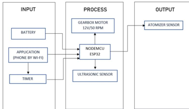
**Figure 8: Block Diagram of Automated Fumigation device**
