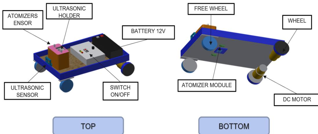
**Figure 6: Development of mechanical and electrical components for Automated Fumigation device**
