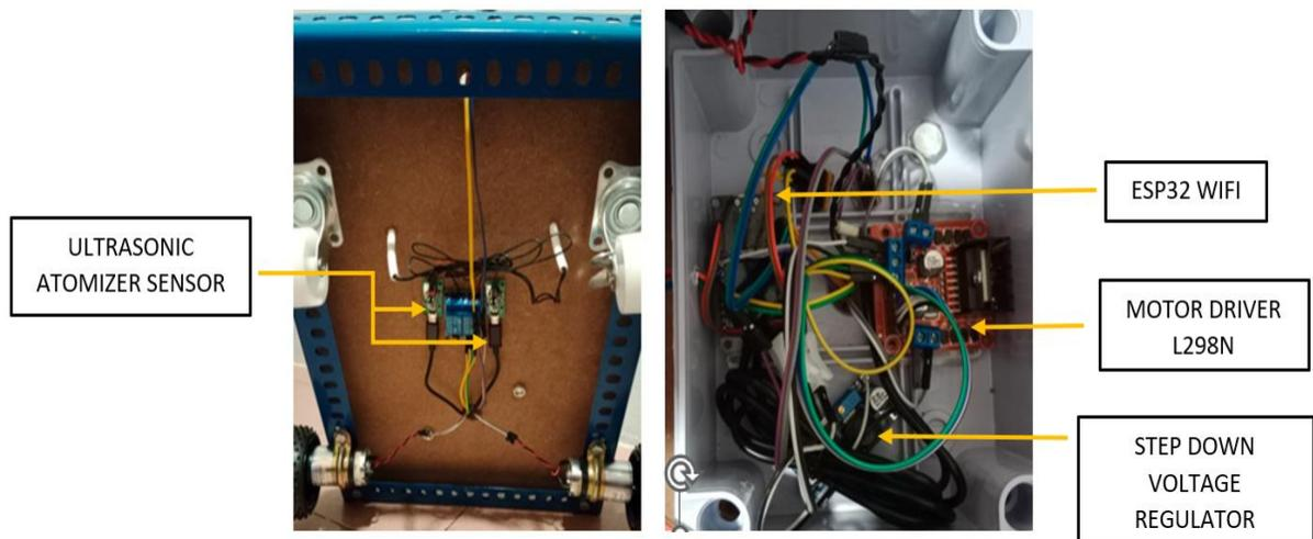
**Figure 5: An Automated Fumigation device circuit installation**
