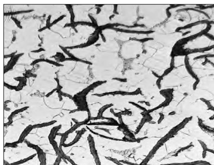
Figure 5.1: Photomicrograph of Grey iron: the dark graphite flakes are embedded in an -ferrite matrix
