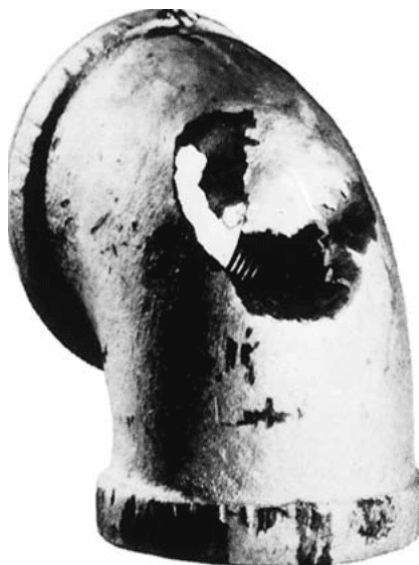
Figure 7.23 Impingement failure of an elbow that was part of a steam condensate line.
