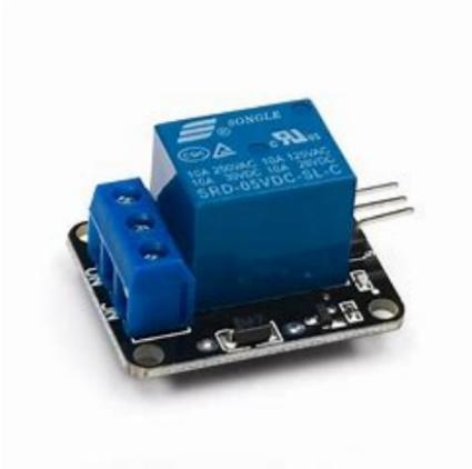
Relay modules (or power relay modules) are ubiquitous electronic components. They are an exceedingly significant component of any home automation project. You will require a relay module if you use a low voltage microcontroller such as an Arduino to control motors or lighting circuits.
