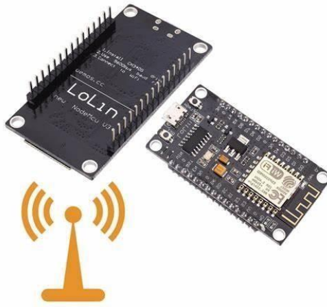
Figure 3.9 ESP 8266 serial Port wifi
