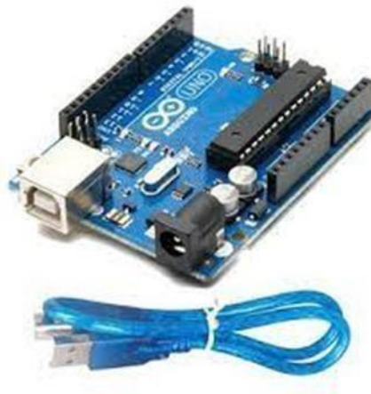
Figure 3.5 Arduino Uno R3 Compatible (CH340G)
