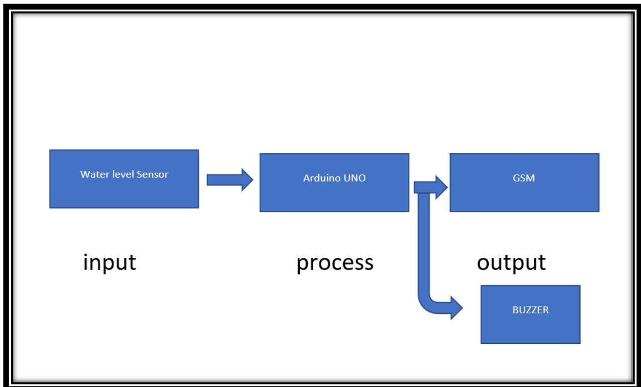
A block diagram of a remote flood monitoring system is displayed. Input, control system, and output are the three sections of this block diagram. A water level sensor and a water flow sensor are included in the input area. The major controllers are the Arduino Uno and the GSM module, while the outputs are the buzzer, LCD, LED, and phone.
