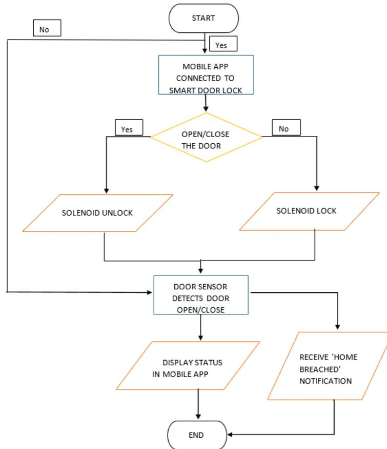
Figure 3. 1: Flow chart of operation of the system
