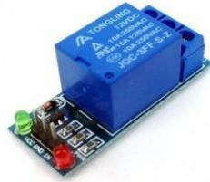
Relay Module is an electrically operated switch. It is responsible for completing the connection of solenoid lock and the power supply.
