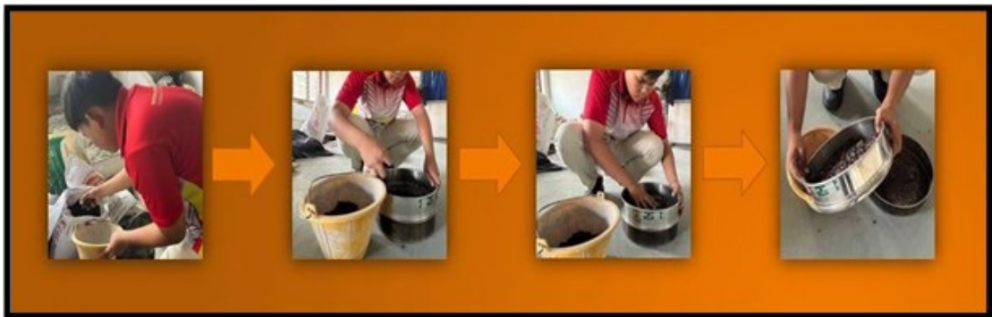
Rajah 10: Prosedur Ayakan Tempurung Kelapa Sawit
