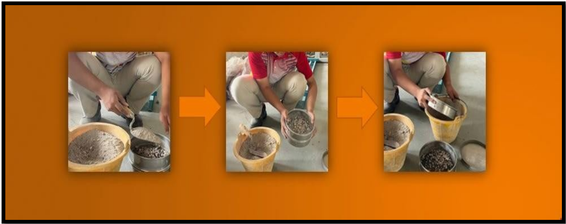
Rajah 11: Prosedur Ayakan Agregat Halus
