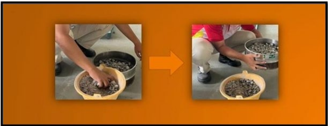
Rajah 12: Prosedur Ayakan Agregat Kasar
