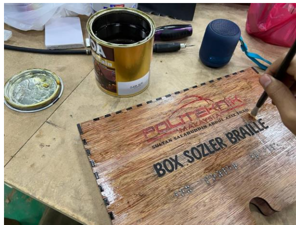
Figure 3.6 (g) : Brush cover Box Sozler Braille with clear liquid
