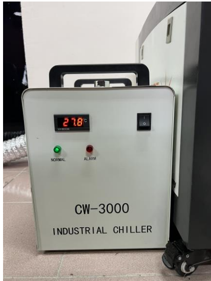
Figure 3.5 (b) : Industrial Chiller switch on
