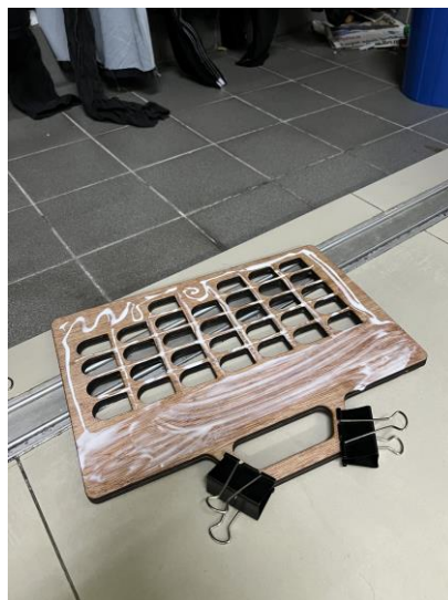
Figure 3.6 (c) : Glue the pieces of wood using wood glue
