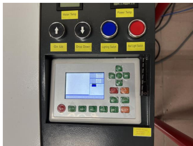
Figure 3.5 (k) : Button control Machine CO2 Laser Engraving
