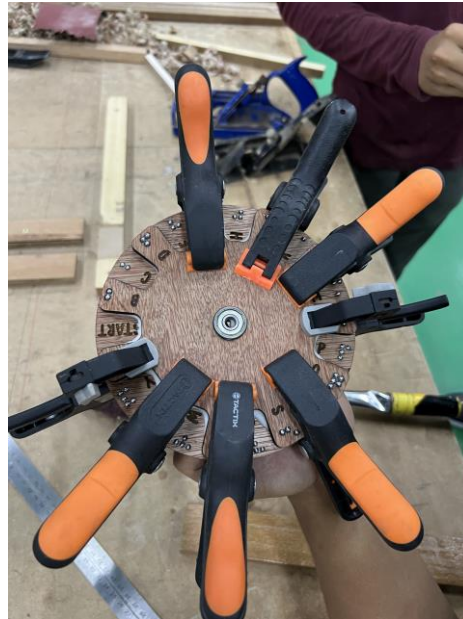
Figure 3.6 (h) : Clamp the part of Wheel Sozler Braille
