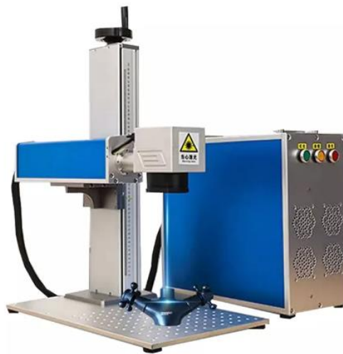
figure 2.3.2 (b) : Laser engraving machine where the X-Y table stationary, only laser is moving.
