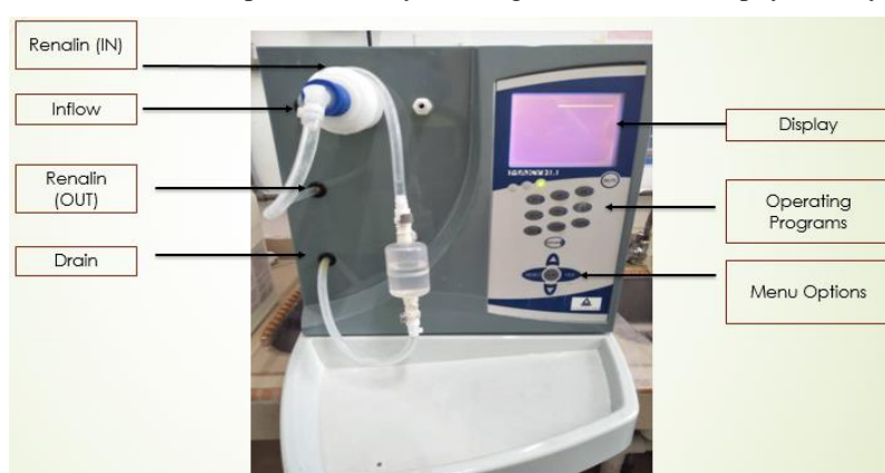
Figure 7.6: Physical layout of Maky 21.1
