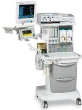
Figure 4.1: Design of modern anaesthesia machine.
