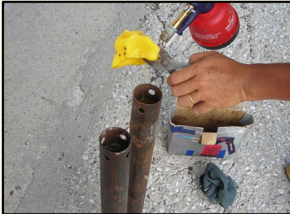
Figure 19 : Applying Melted Paraffin to seal soil sample
