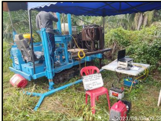
Figure 10 : Cone Penetration Test
