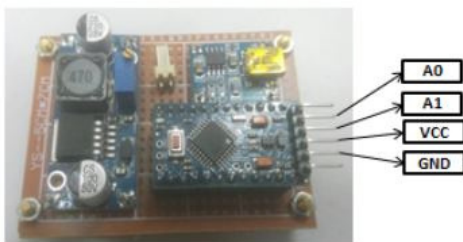
Figure 2: Arduino circuit have been used to simulate the data from the FSR sensor
