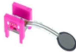
Figure 3: FSR sensor that use for Auto walker to get the analog reading
